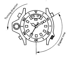
The register ring can be turned only in the counterclockwise direction. An anti-reverse mechanism with a click sound is provided in order to protect the above mechanism, do not use excessive force in turning in the clockwise direction. Set the triangle mark ( $\blacktriangle$ ) to the position of the Minute Hand at the dive start time to read the elapsed time. The ring can be turned in units of every 0.5 minute.
