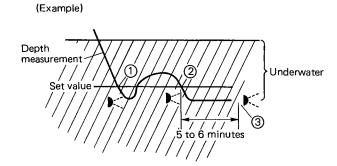
When the diving depth exceeds the previously set value, a buzzer sounds from 1 min. to 1 min. 10 sec. The buzzer stops sounding when the diver goes up toward the water surface beyond the set value.
